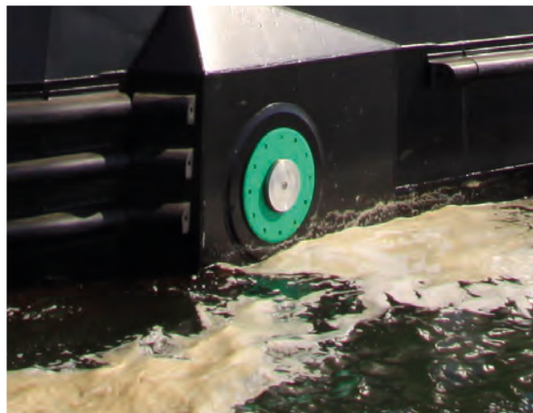
Coupler unit seen from the Port side bow of the pusher.
